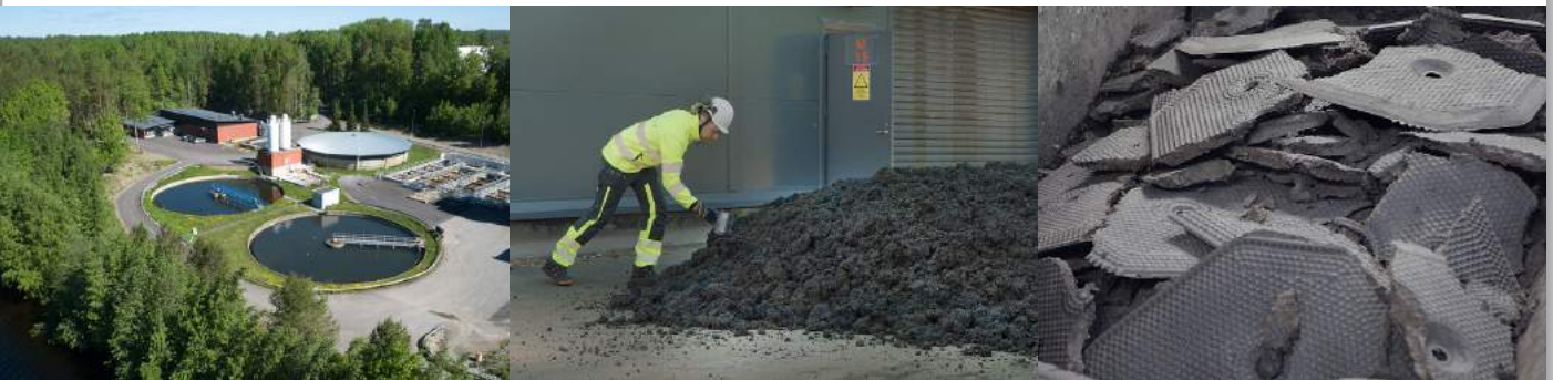
Municipal sludge trial in Heinola: the municipal wastewater treatment plant produces sludge that is converted into hydrochar by C-Green's biorefinery
