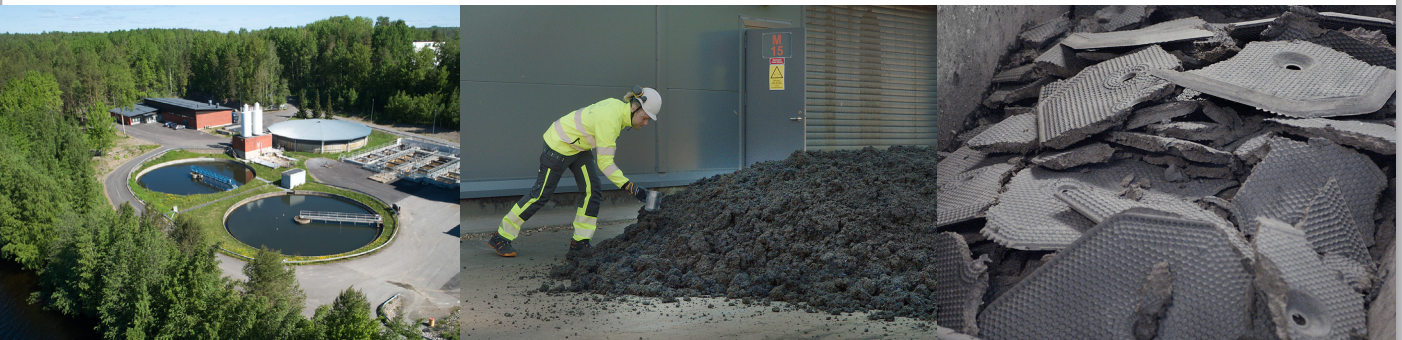
Municipal sludge trial: the municipal wastewater treatment plant in Heinola produces sludge that can be converted into hydrochar by C-Green's biorefinery
